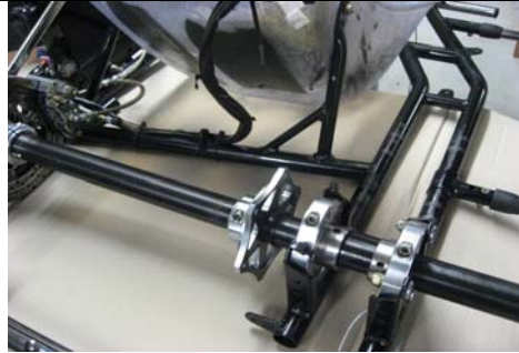
Your chassis must have a sprocket carrier inside for left drive engines
