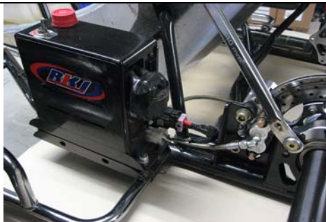
Put battery in battery pack and mount the pack on your chassis
