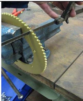
Make sure you cut the right way ( in between 2 teeth and not touching a mounting hole)
