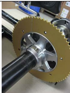
Fix sprocket to sprocket holder with using all 6 fixing holes
