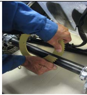
Easy way to get sprocket on inside sprocket carrier
