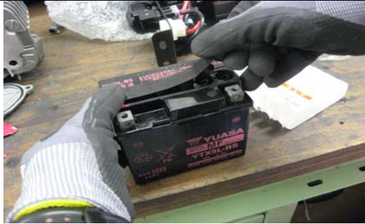
After filling close battery with closing strip
