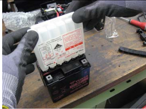
Fill battery with enclosed battery fluid
